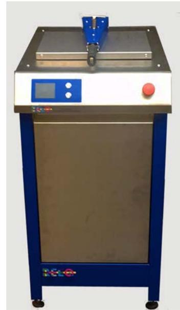
Filling cartridges is a precise job and can take a lot of manual labour. Our new filling machine REEQ CF700-SA is a semi-automatic filling machine. With the basic model, you can fill 24 black or 8 colour cartridges.
